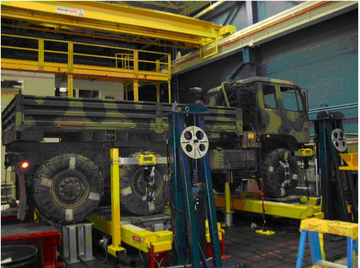
Figure 1: Overall view of the SPiDER being used to test a 3-axle vehicle. The axle frames are under the first and second axles. The third axle is on a wheel stand. For this setup, only the first axle is being test
