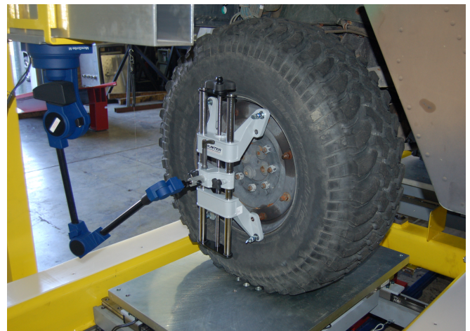
Figure 3: The coordinate measuring machine used to measure wheel motion in the x-, y-, and z-directions, as well as the steer and camber angles. A commercially made alignment fixture is used to adapt the stylus of the measuring machine to the tire rim, and the alignment fixture automatically finds the centerline of the tire.
